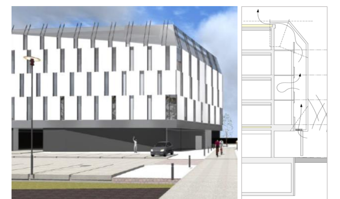
Fig. 8. BIPV façade solution proposed for building A. (Image source: Skanska Norge/Egerdahl&Nordbø.)
